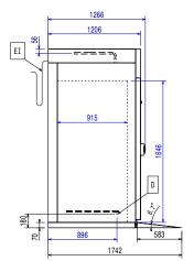
Electrical inlet (power) ΕI Refrigerant Outlet RO
